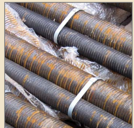
ASTM A722 grade 150 threaded anchor bars used with pipe pockets
