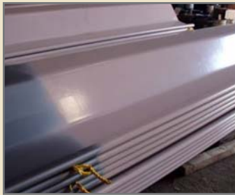
Coated sheet pile staged for delivery
